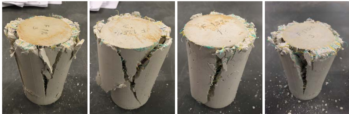
(e) Cylinder after compression test. 1.00% fibre concentration. (f) Cylinder after compression test. 1.25% fibre concentration. (g) Cylinder after compression test. 1.50% fibre concentration. (h) Cylinder after compression test. 1.75% fibre concentration.
