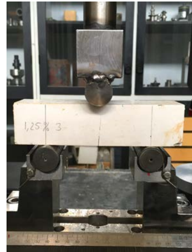
(c) Picture of the set-up used for three-point bending of the prisms.
