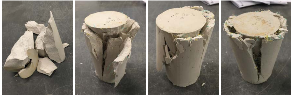
(a) Cylinder after compression test. Reference specimen with no added fibres. (b) Cylinder after compression test. 0.25% fibre concentration. (c) Cylinder after compression test. 0.50% fibre concentration. (d) Cylinder after compression test. 0.75% fibre concentration.
