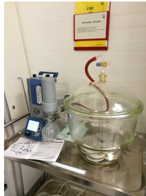
(b) The desiccator connected to the vacuum pump.
