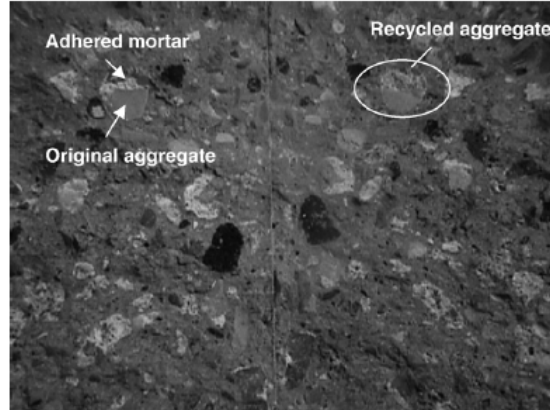
Figure 2.2: NA with attached mortar, taken from [Etxeberria et al., 2007].
