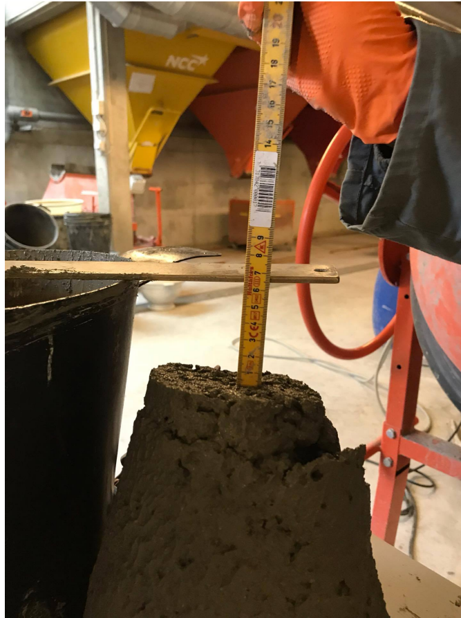
Figure 3.2: Slump test with the mix design B
