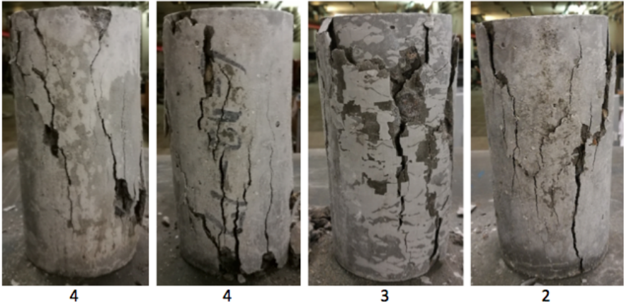
Figure 2.25: RCA20% (4-8mm), 28 days, X
