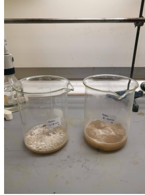
(b) Nitric acid reacting with the attached mortar.
