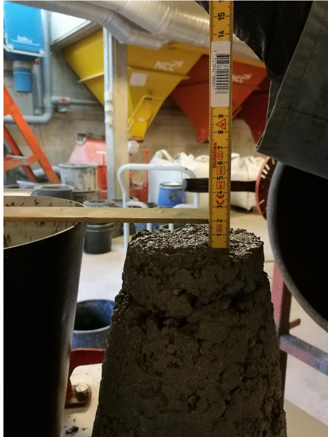
Figure 3.1: Slump test with the mix design A
