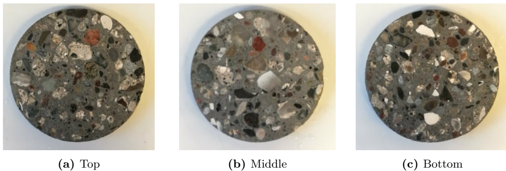
Figure 5.19: Cut discs for the RCA50% specimen
