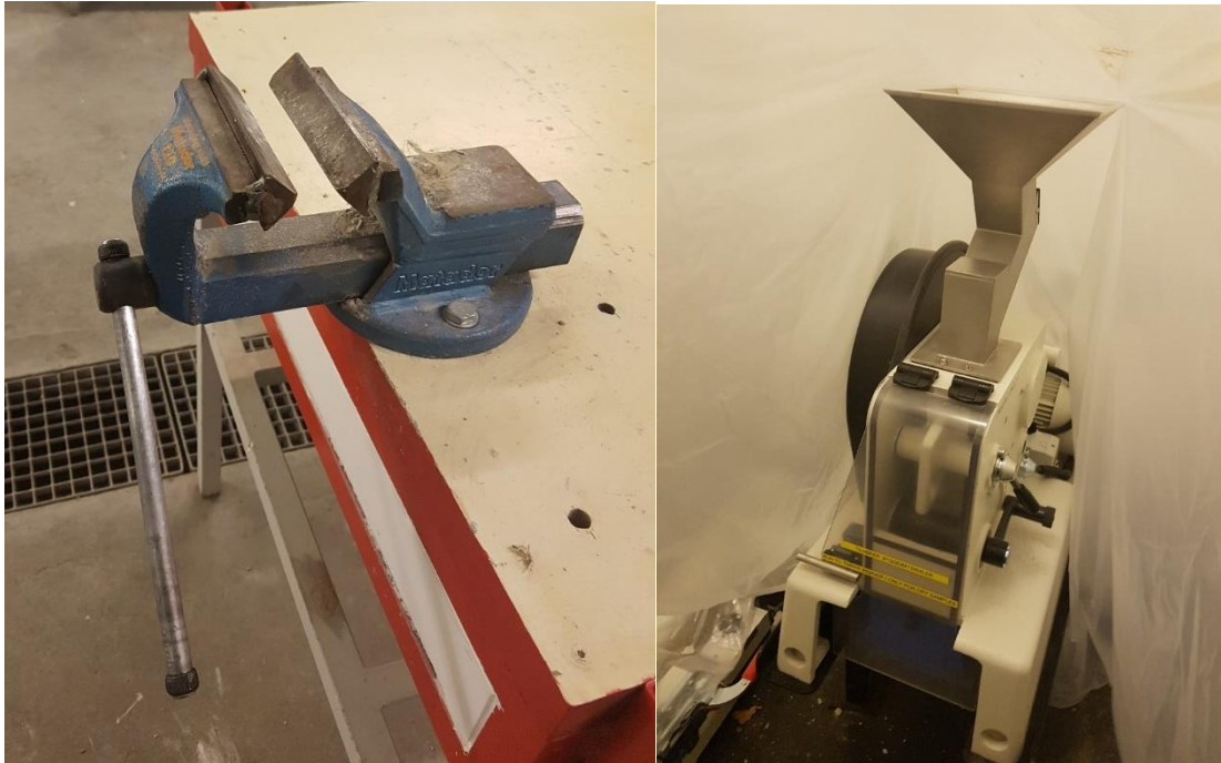
Figure 3-2 Vice with triangular beaks and crushing machine from Buch and Holm
