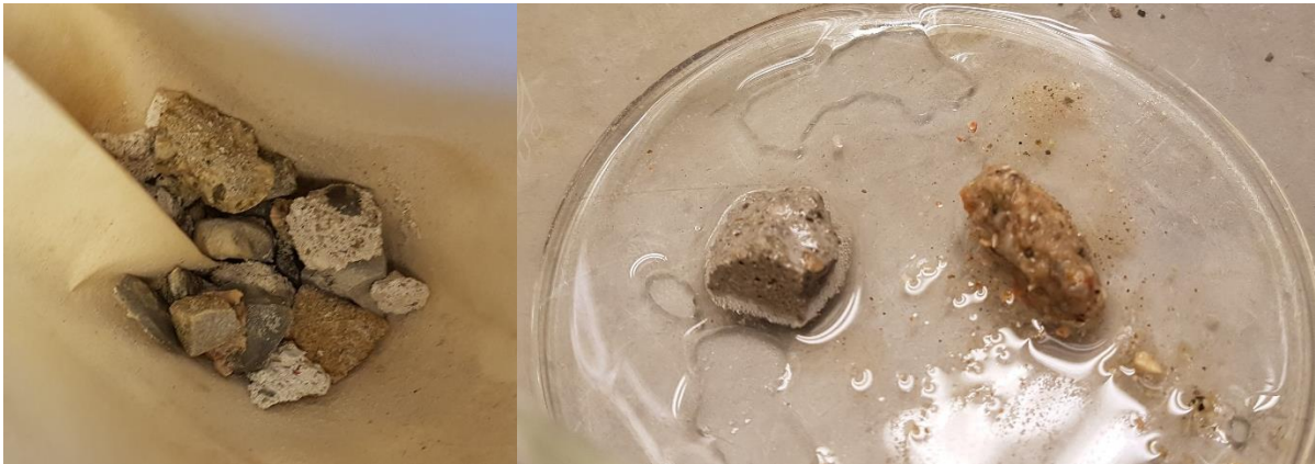
Figure 4-1 RCA after testing for cement paste content (left) and unknown substances tested with nitric acid (right)
