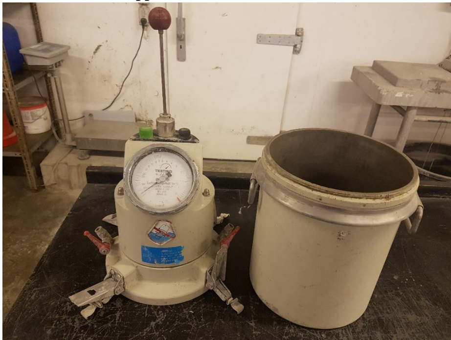
Figure 3-12 Apparatus to access air content in wet concrete
