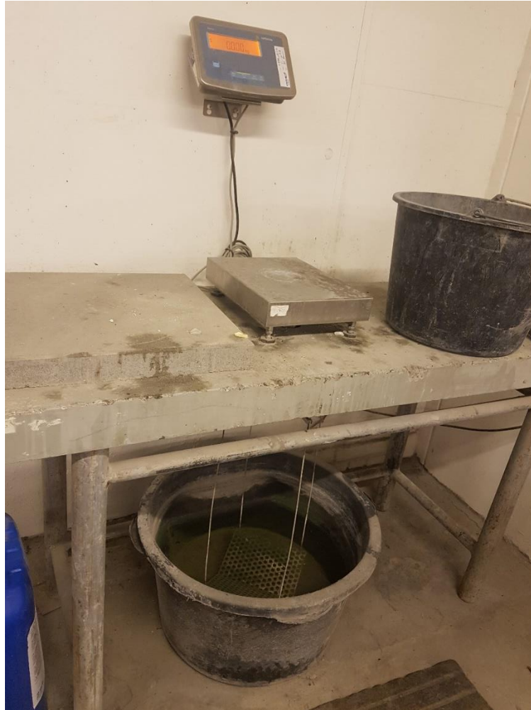
Figure 3-14 Set up in workshop to weight the cylinders above and below water
