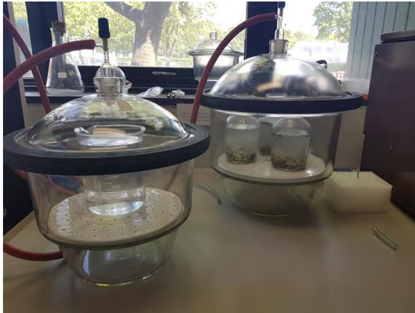
Figure 3-4 Vacuum containers for the pycnometer test (Herløv 2017)
