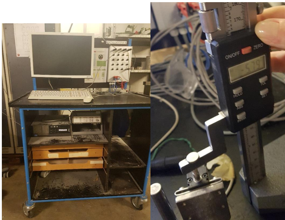
Figure 3-16 The Data Logger (left) and the ruler used for calibration (right)
