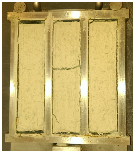
Figure 4.4: Cracked specimens after drying in 48 hours under 50^{\circ}\text{C} .
