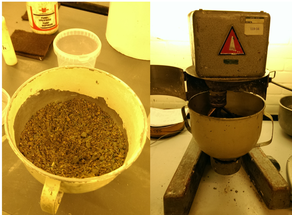
Figure 4.2: The mixing process. Left: Dry mixture (clay, gravel and fibers). Right: Mixing in Toni, industrial mixer
