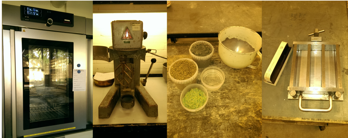
Figure 4.1: Components to be used for mixing and casting. Left: Oven - Memmert UF 160. Left center: Toni, industrial mixer. Right center: Materials and industrial mixing bowl. Right: Specimens and compression piston.
