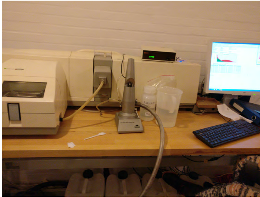
Figure 3.5: The laser diffractometer, Mastersizer 2000, used to create grain-size distribution curves for the smaller aggregates.
