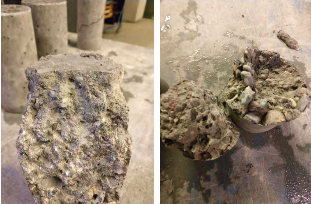
(a) The specimen from the second B2 casting with the lowest compressive strength. (b) A specimen from the second B2 casting with fracture through mortar and not through aggregates.
