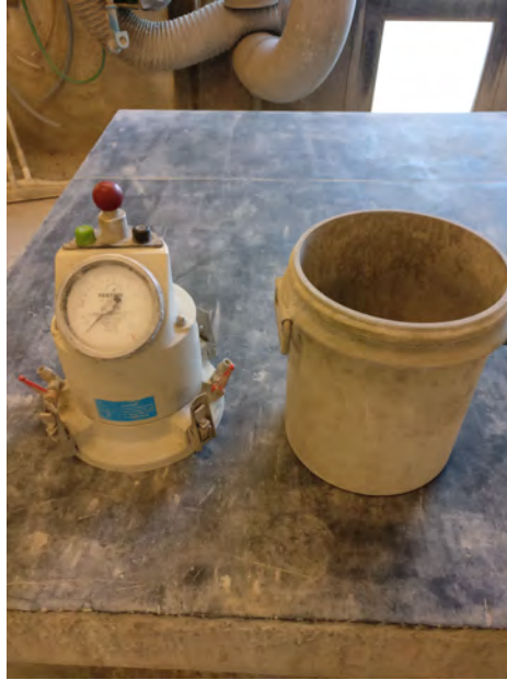
Figure 3.9: Pressure gauge used to measure the air content.
