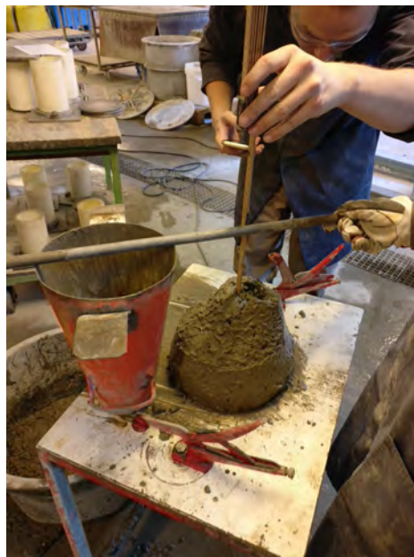
Figure 3.8: Measuring of the slump.
