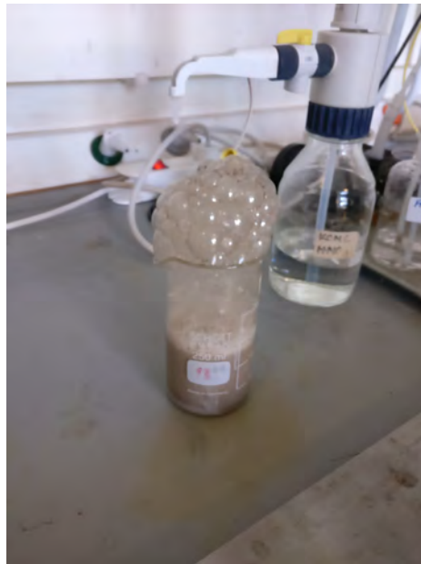
Figure 3.3: The RCA reacts with acid during the attached mortar experiment.
