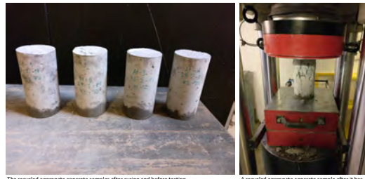
The recycled aggregate concrete samples after curing and before testing.
