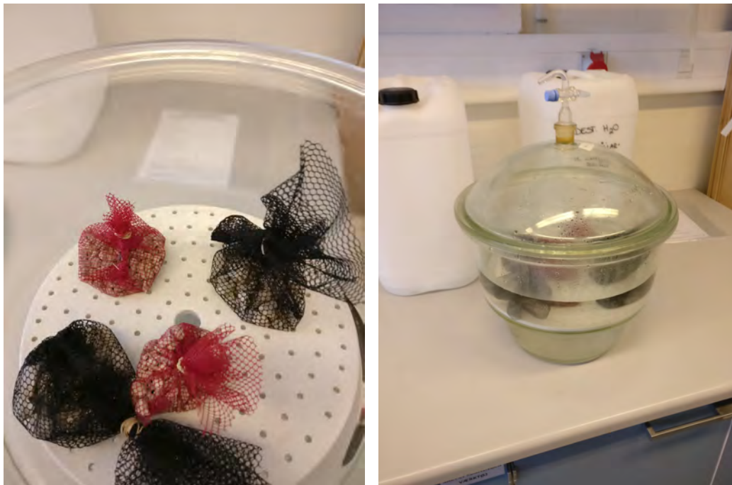
(a) The aggregates placed in nets. 4-8 mm in red nets and 8-16 mm in black nets.
