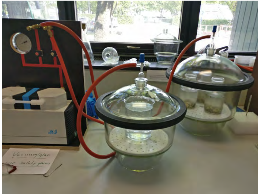
Figure 3.2: The pycnometer experiment. The pycnometers are placed in the desiccator in the back. In the desiccator in the front there is a glass of water.
