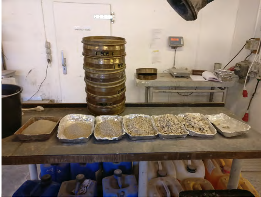
Figure 3.4: The sieves used to perform the sieving experiment. The aggregates can be seen in front of the sieves, going from small aggregates to the left to large aggregates to the right.
