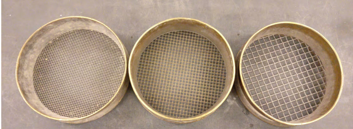
Figure 3.6: The three sieves used. From left to right: 4 mm, 8 mm and 16 mm.
