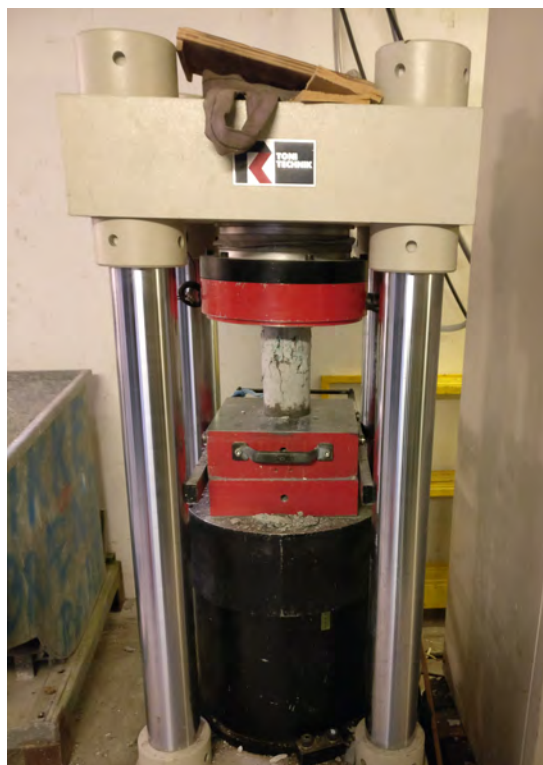
Figure 3.10: The test machine and a test specimen after compression test.
