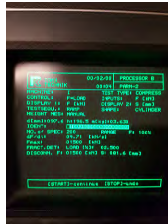
(b) The display to edit the test values such as pressure rate and fracture rate.
