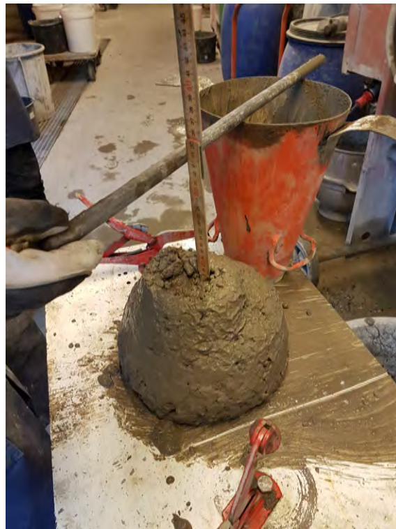
(b) Slump test in practice.
