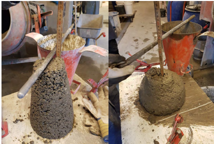
Figure 2: The difference in slumps depending on the mix design. Left picture shows mix design B7 with a slump of 5mm and the right picture shows mix B1 with a slump of 130mm. There is clearly a huge difference if the aggregates are dried in the oven or simply surface dry.
