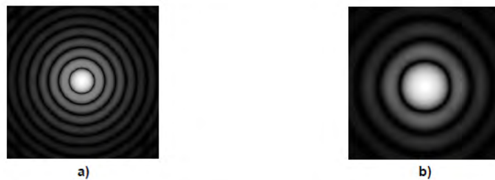
Figure 3.7: The patterns created by 2 different spherical particles. The scattering pattern a) is twice as large as b). Found in DS-ISO13320 2009.
