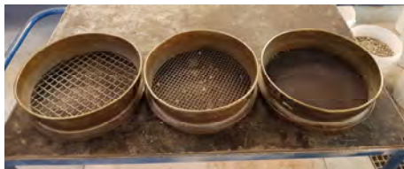
Figure 2: Sieves used to divide aggregates into 16-8mm and 8-4mm fractions. (From left: 16mm, 8mm and 4mm)
