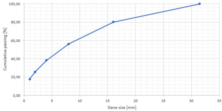
Figure C.2: Sieve column 1 (1-31.5 mm).
