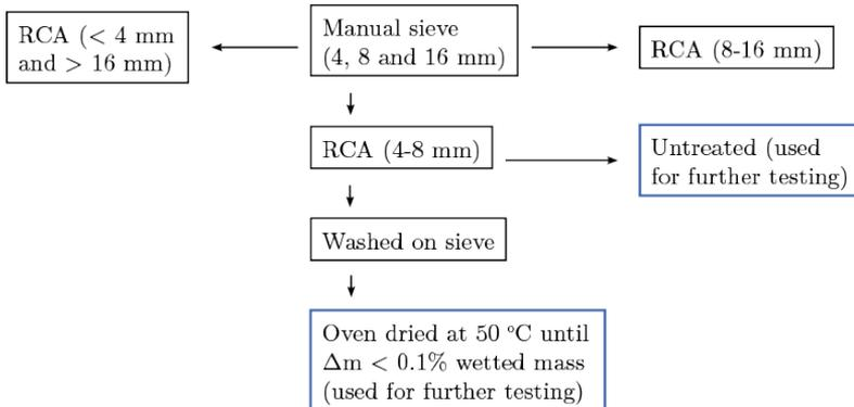
Figure 3.2: Preparation process.
