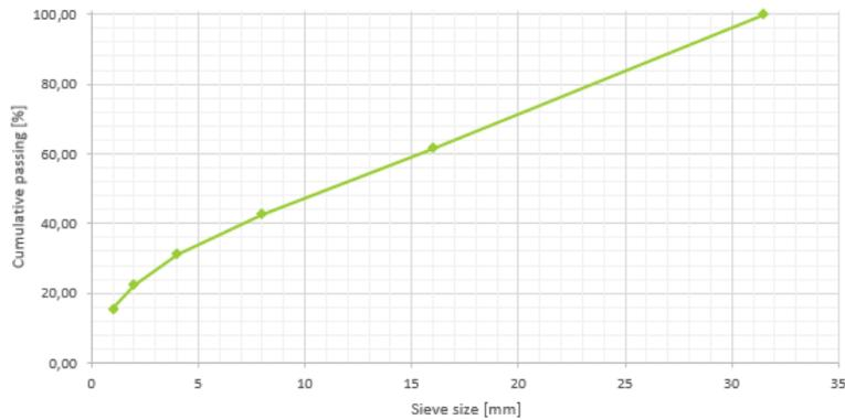
Figure C.4: Sieve column 2 (1-31.5 mm).
