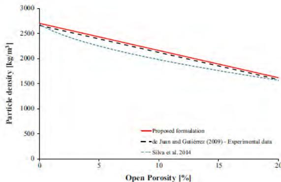
Figure 2.9: Proposed correlations for the physical properties of RCAs (Pepe 2016). Results of RCA (4-8 mm) are illustrated green.
