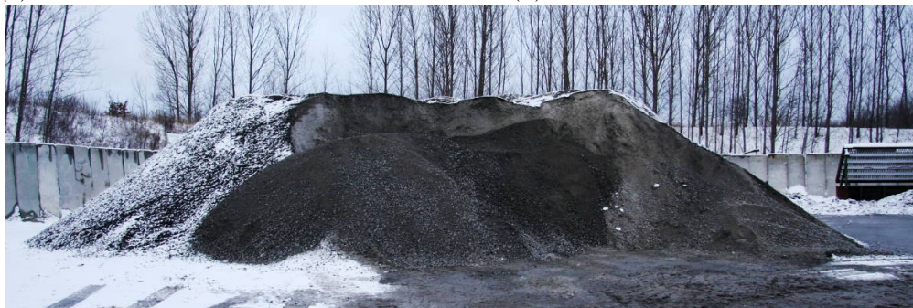
(c) Concrete waste after crushing
