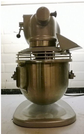
Figure 4.1: Hobart Mixer used to mix the mortar mixture.
