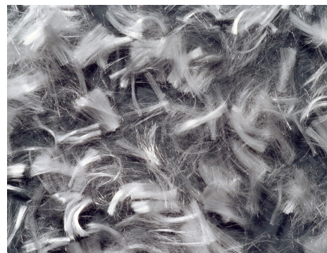
(b) Micro Fibre called Fibrin Fiberflex
