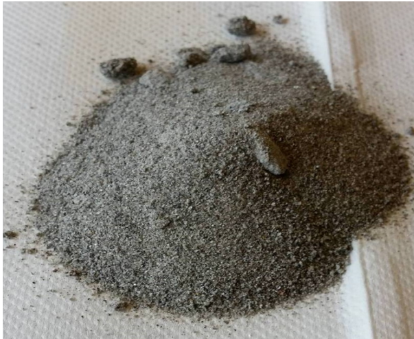
Figur 5.1: Zinkgruvan mine tailing
