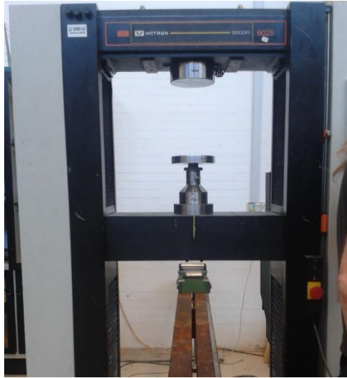
Figure 7-17 - Machine used to test the compressive strength of the samples
