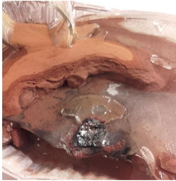
Figure 15-1 - Broken glass jar and microwave plate. The ash and plate is wet in an effort to cool it down.
