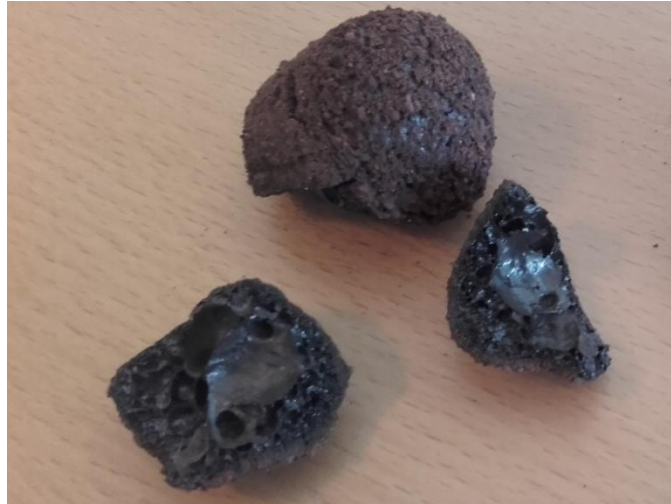
Figure 12-1- LWA 0-2 sintered together
