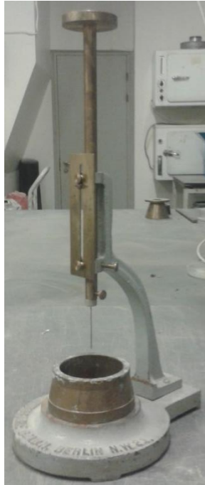
Figure 7-7 - Vicat apparatus used in this project
