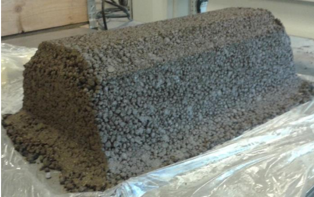
Figure 7-10 - block made in the block machine
