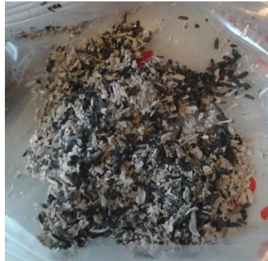
Figure 7-1 - Larger pieces of ash, after 1 hour at 550° C. The black parts are unburned
