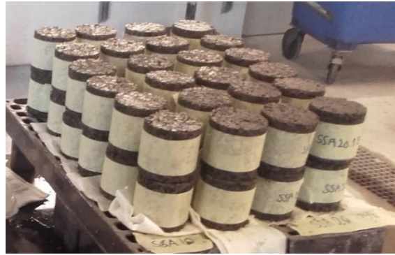
Figure 7-15 - Cores cut into multiple samples
