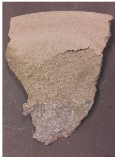
Figure 7-3 - Piece of the bottom ash, brown on top, gray on the bottom
