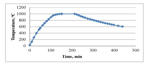
Figure 4: Corresponding heating and cooling profile versus time in the furnace.
