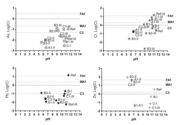
Fig. 5. Summary of the results from the leaching test of the untreated and treated ashes at L/S 2, where C [mg/l] is the concentration of each element in the leachate, in order to assess the environmental impact according to Danish regulations for landfill (FA1 and MA1) and recycling (C3).
