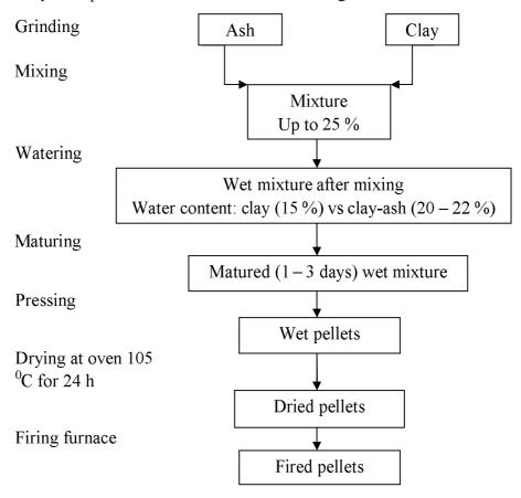
Figure 2: Brick pellet making processes.
