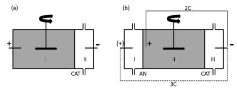
**Fig. 1.** Experimental setups: (a) two-compartment cell (2C); (b) three-compartment cell used for 2-step EDS treatment in Experiment B3: first 2C, effective two compartment cell by current passing through the anode in the ash suspension and the cathode; and then 3C, effective three compartment cell by current passing through the two electrodes in electrolyte solutions (dotted route). AN, anion exchange membrane; CAT, cation exchange membrane.
