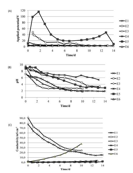
**Fig. 2.** Development of voltage between the working electrodes (A), development of pH (B) and conductivity (C) of the ash suspensions within the first 14 days of EDR treatment. In this period of time the changes were considered significant.
