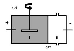
Fig. 1. The schematic drawing of the types of EDR cells used in the experiments. Anion exchange membrane = AN; cation exchange membrane = CAT.
