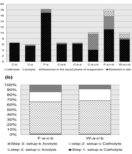
Figure 1. Arsenic extraction and transport during EDS treatment. (a) Distribution of the total mass of As in the EDS cell at the end of the experiment: where As dissolved in liquid solution includes electrodes in ash suspension (assumption: ionic As species moved and deposited on electrodes), stirring, solvent (water); and (b) Contribution of each treatment step to the total extraction.
