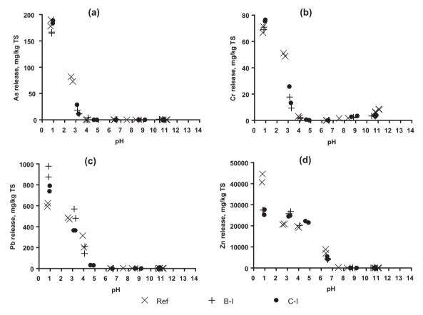
Fig. 4. The dependence of each element in the raw Ref ash and the washed ashes B-1 and C-I available for release (mg/kg TS) into nitric acid solutions with different pH values: (a), As; (b), Cr; (c), Pb; (d), Zn.
