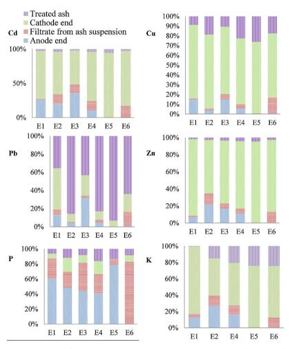
**Fig. 3.** Distribution of elements in the electrodialytic cell after remediation. Anode end includes element at the anode, in the anion-exchange membrane and in the anolyte. Cathode end includes the element at the cathode, in the cation-exchange membrane and in the catholyte. Elements in the treated ash were measured on dry basis. Due to the bad mass balance of K resulting from pump leaking, the distribution of K in E3 was not given.
