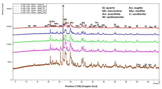
Figure 6: Mineralogy of the fired bricks.
