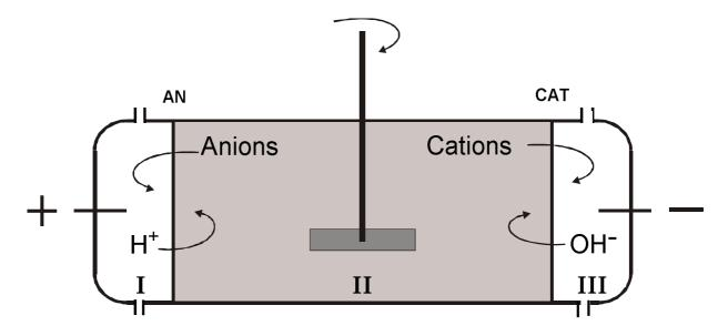
Figure 1: The princple of EDR treatment and the schematic drawing of a 3-compartment EDR cell. AN - Anion exchange membrane, and CAT - cation exchange membrane.
