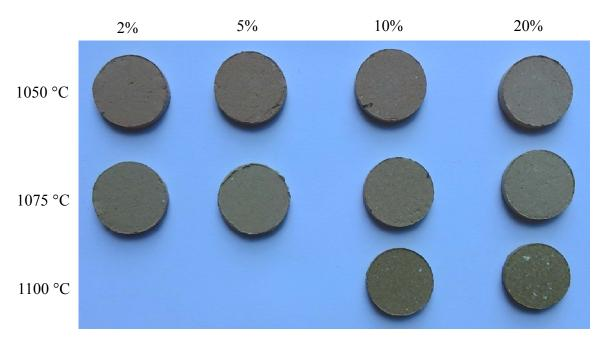
Figure 2. The appearance of the pellets having different ash contents and fired at different temperatures.
