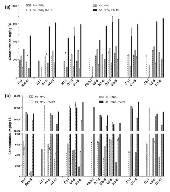
Fig. 2. Total concentrations (mg/kg total day solid) of the heavy metals in the ash samples: (a) results for As and Cr; and (b) results for Pb and Zn.
