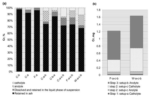
Figure 5: Chromium extraction and transport during EDS treatment. (a) Distribution of Cr, in %, in the EDS cell at the end of the experiment: where Cr dissolved and retained in liquid solution includes electrodes in ash suspension (assumption: ionic Cr species moved and deposited on electrodes), stirring, solvent (water); and (b) Contribution of each treatment step to the total extracted mass.
