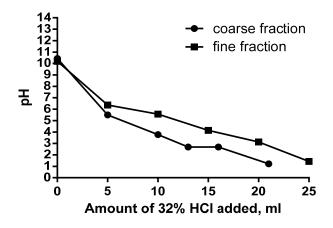
Figure 3: The buffer capacity of the washed fly ash: fine fraction and coarse fraction.
