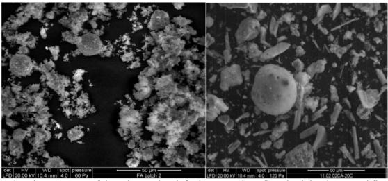
Figure 2: Microstructure of the ash samples: left, the raw MSWI fly ash; right, the treated fly ash by combined water washing and EDR.
